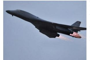
towards us fast. It was a B-1 bomber with wings swept back. The B-1 can sweep its wings back for high speed flight, and they use south east Colorado as a training area for high speed ground-hugging flights.
